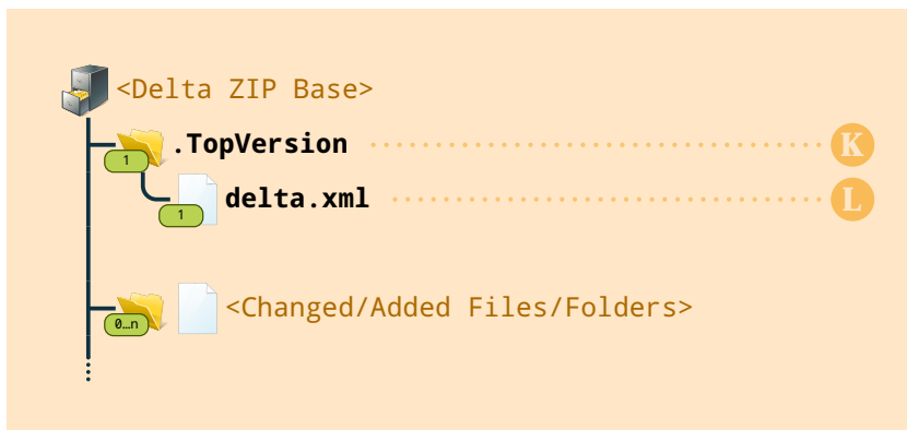
Illustration 3 The structure inside of a delta package.
