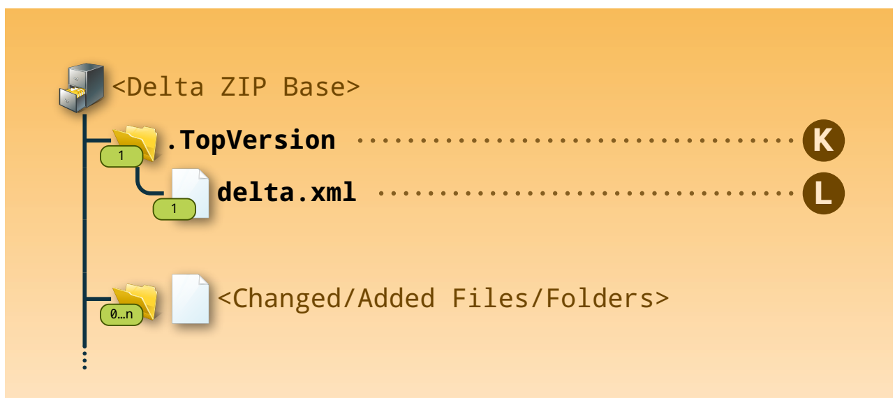
Illustration 3 The structure inside of a delta package.
