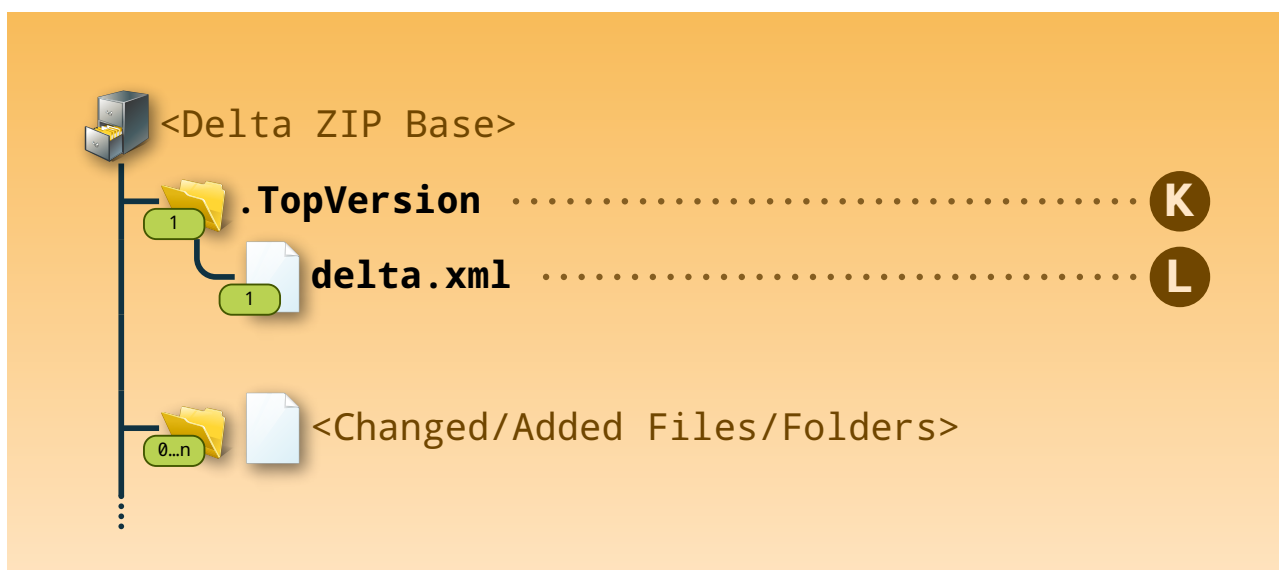
Illustration 3 The structure inside of a delta package.
